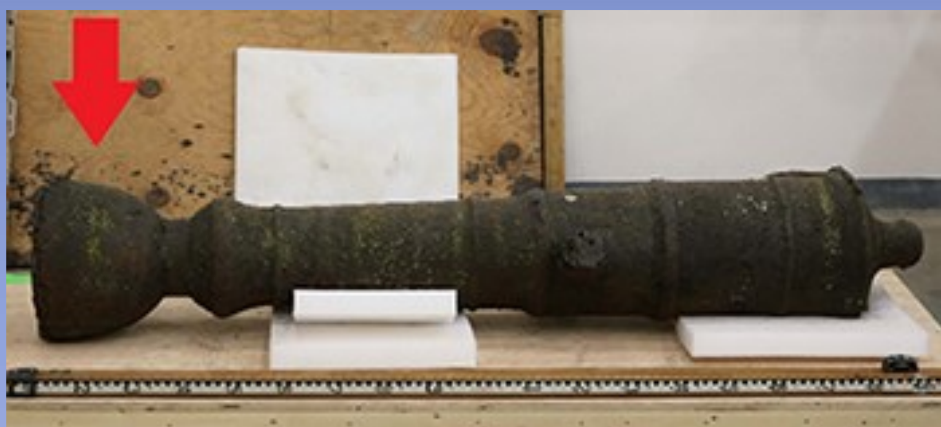
Figure 2: The Mt. Aetna cannon before treatment (arrow indicates the sprue).
